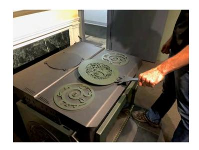
3. Lift the top lid and remove the radiator. The radiator shrouds the catalytic combustor.
