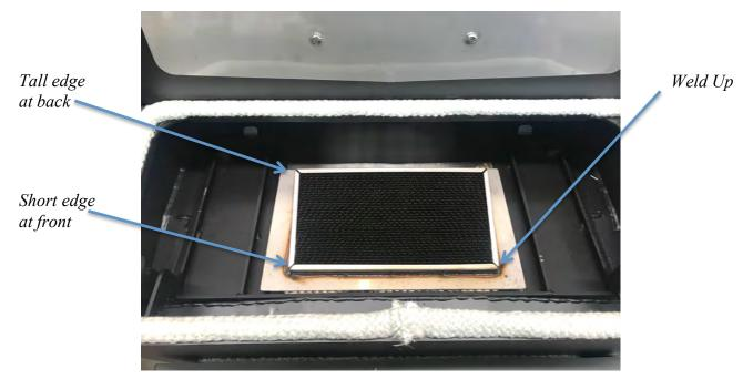
9. Replace the radiator. The standoffs will go towards the back of the stove, and the radiator shield attachment will be at the front of the stove.
