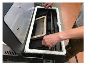
7. Place the new sled into the stove making sure the sled hooks attach to the bypass rod. The hooks will be on the outside of the two round washers welded onto the bypass rod.
