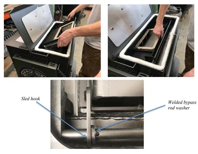
8. Install the combustor. Make sure the weld around the perimeter of the stainless steel flange is facing UP. The flange is welded around the combustor at an angle. The combustor should be installed so the face is directed forward with the short edge at the front, and the tall edge at the back. This position directs the heat produced by the catalyst forward.
